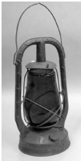
The “Merribrooke melter” was the name given to the modified lantern Morris used to pour paraffin wax on grafts.
