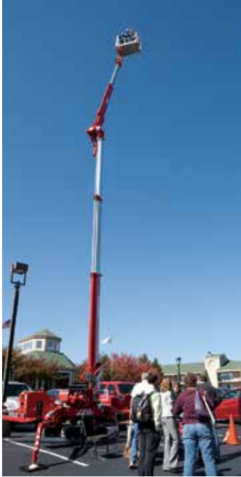
Two TACF members really got a lift out of the Summit. Teupen Corporation brought one of their remarkable Leo 23GT Aerial lifts, which has the capacity to raise passengers 75 feet in the air.
