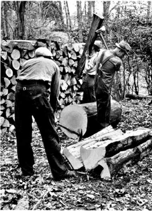
Within a radius of one hundred miles from the Champion mills the chestnut trees are cut into logs, barked and split, to be trucked to railroads for shipment to the mills.
