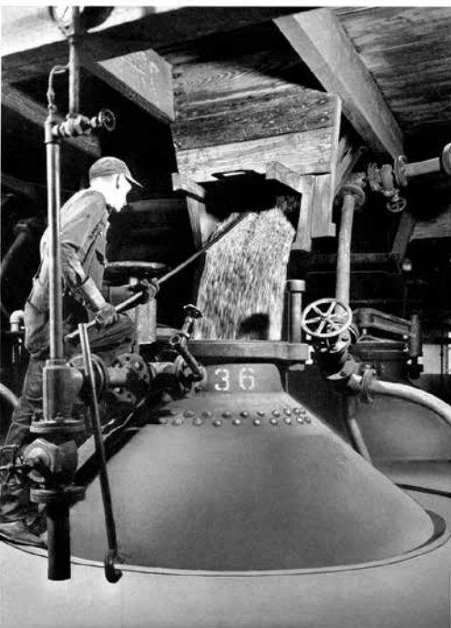
A gate opens and a deluge of chips falls from bins above. Nearly five-hundred cubic feet fill each autoclave with a fresh loading approximately every forty minutes.
